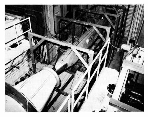
IN SANDIA'S LIGHTNING SIMULATOR, an Air-Launched Cruise Missile was subjected to direct strokes of severe lightning, part of a joint Atmospheric Electricity Hazards Protection program.
